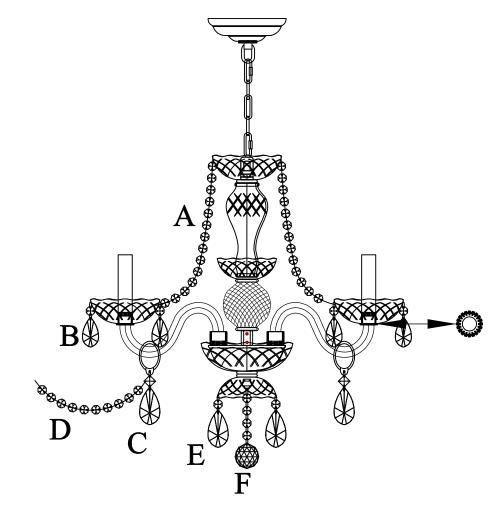
Connect both ends of D with C
